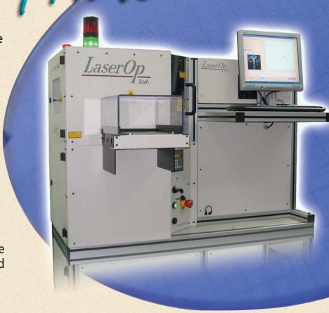
Integration into production lines: A short conveyer propagates the trays through the marking compartment. Just introduce the tray to the entry port and collect it, with marked lenses, at the exit.
